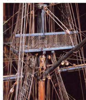
Close-up of the main topsail-yard parrel.
