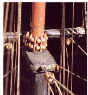
Close-up of the main topsail-yard parrel.
